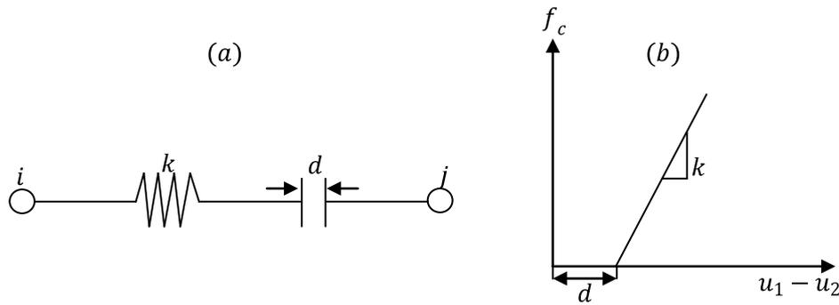
Figure 1. Contact element model, (a) Contact element and (b) behavior of the contact element
