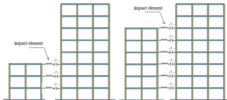
Figure 2. Finite element mathematical model and Elevation view
