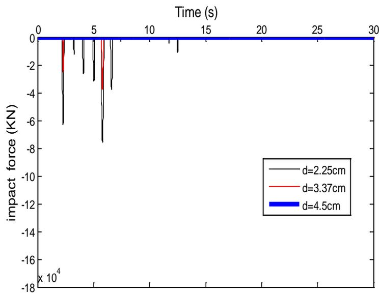
Figure 3. Impact force time history, nonlinear MDOF (8-3) for 50%, 75% and 100% of required gap.
