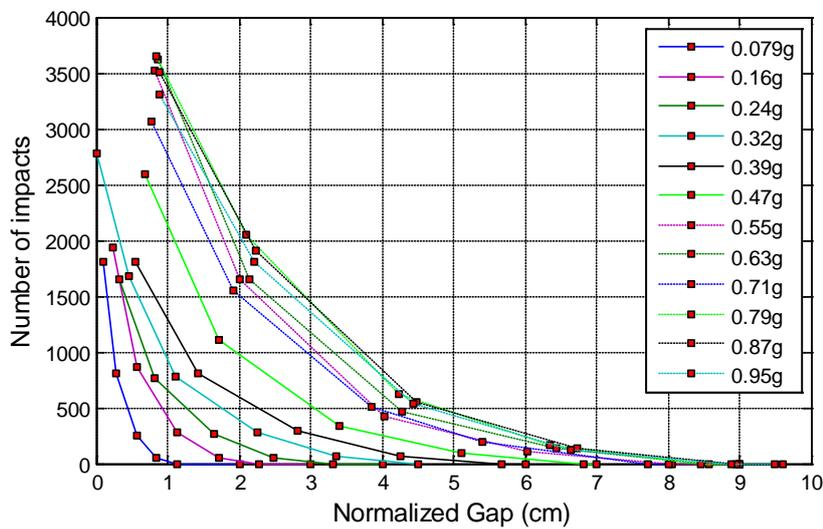
Figure 5. Total number of impacts for adjacent buildings (SP8-SP6) in terms of the size of the separation distance
