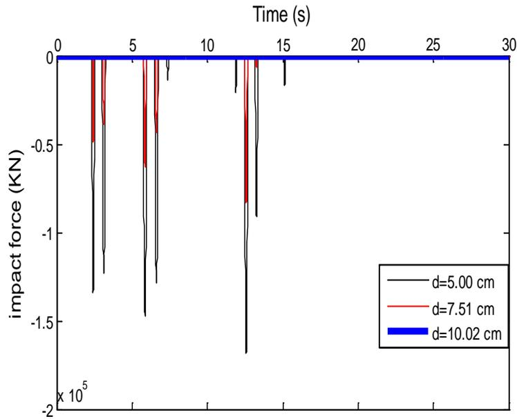
Figure 4. Impact force time history, nonlinear MDOF (8-6) for 50%, 75% and 100% of required gap
