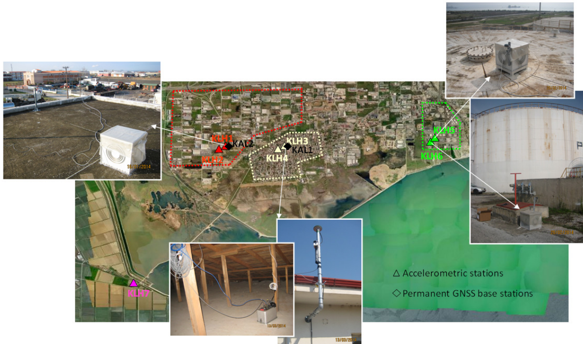
Figure 1. Subdivision of the investigated Kalochori area into three urban sub-zones [i.e. industrial area (red dots), residential zone (yellow dots) and oil tanks zone (green dots)] and locations of the corresponding accelerometric and GNSS base stations.
