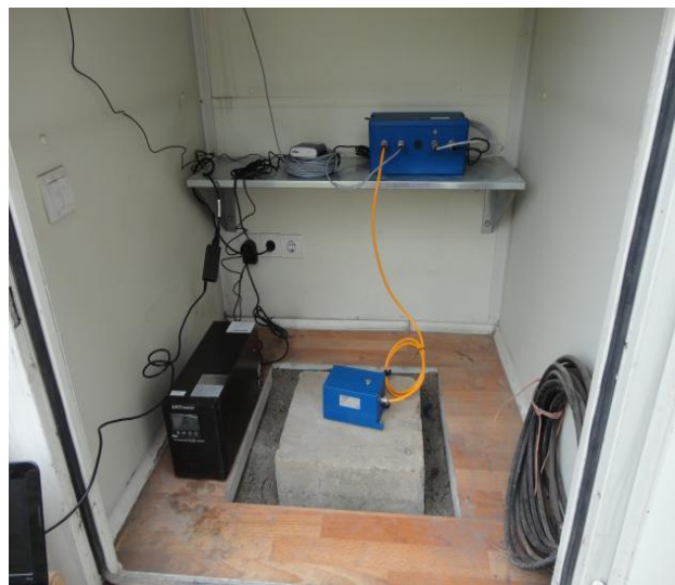
Figure 4. Typical outside and inside view of a strong-motion station.
