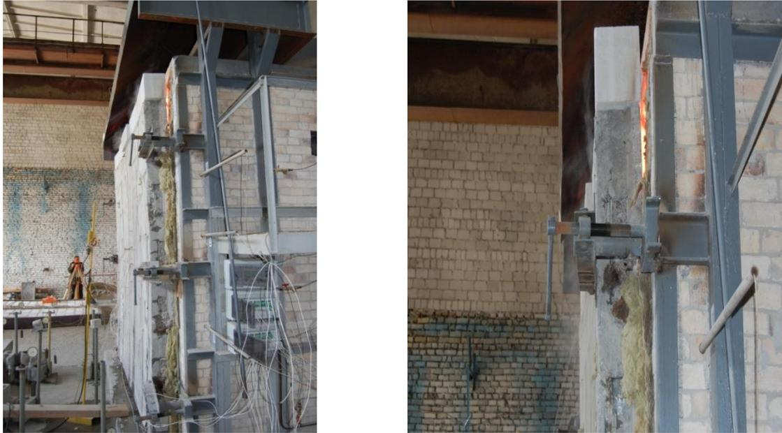
Figure 8. Wall panel BC-111 during the fire test
