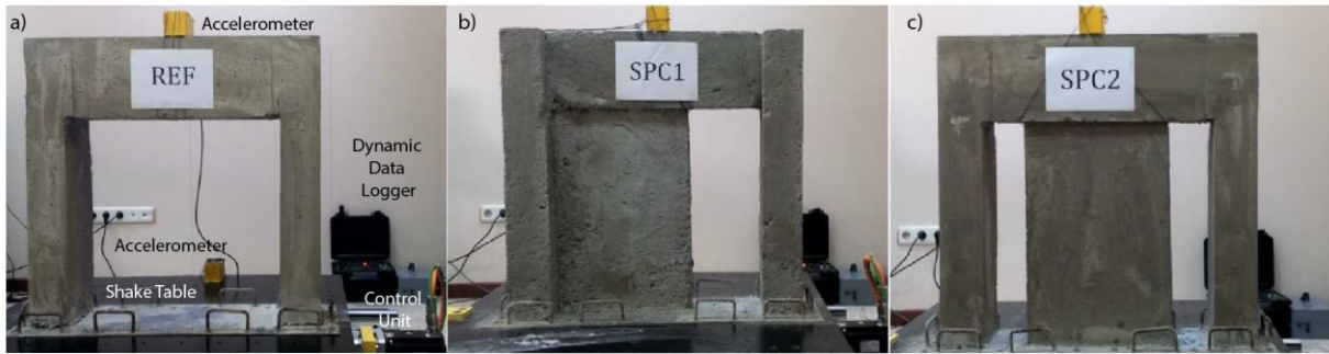
Figure 5. Instrumentation of test specimens and general layout of the test setup
