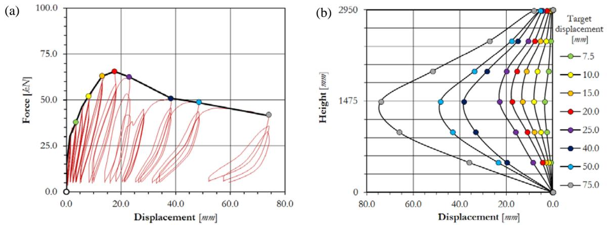
Figure 11. Specimen TA5: (a) Force-displacement response; (b) Deflection along the height
