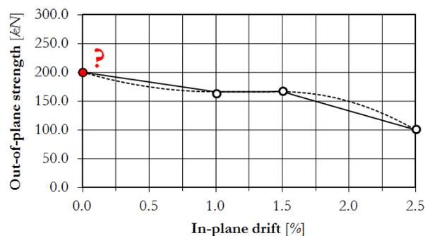
Figure 13. Out-of-plane strength reduction in function of in-plane drift
