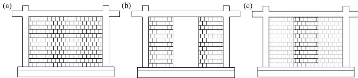
Figure 2. (a) Fully infilled: TA1, TA2, TA3; (b) Partially infilled: TA4; (c) Vertical infill stripe: TA5
