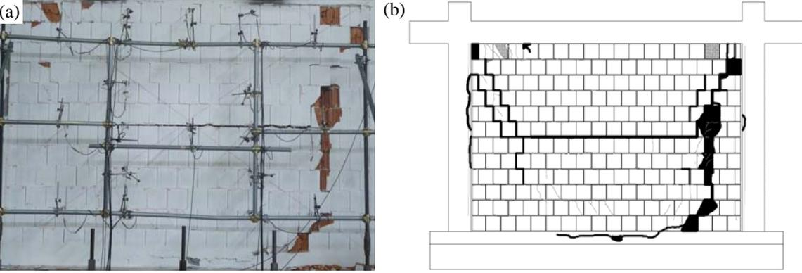
Figure 9. Specimen TA3 (previous in-plane drift: 1.0 %): (a) Damage at  $75\text{ mm}$  target displacement; (b) Crack pattern (in black – out-of-plane damage; in grey – previous in-plane damage)
