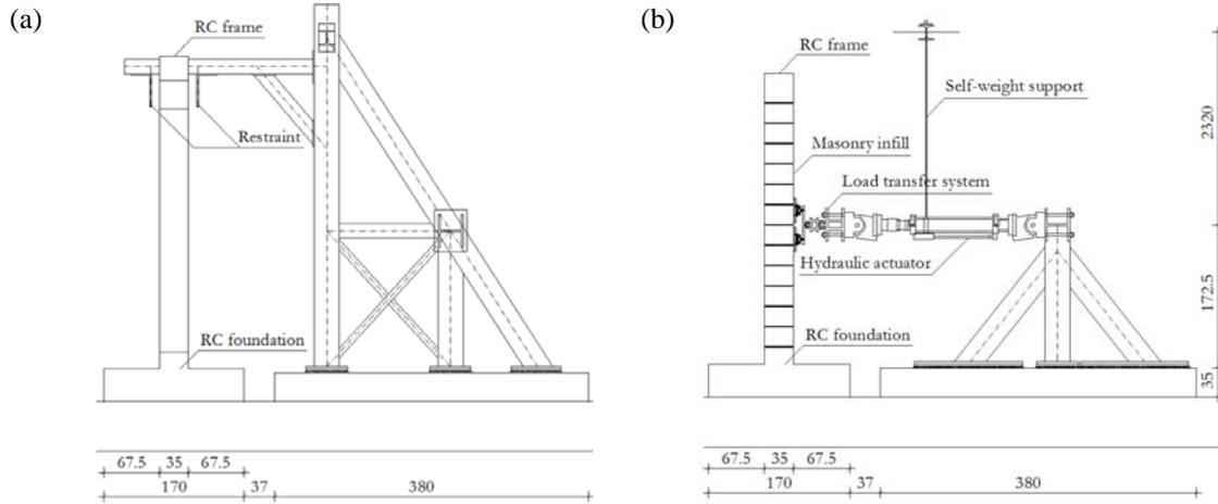
Figure 4. Layout of the out-of-plane test setup: (a) Restraining plane; (b) Reaction plane
