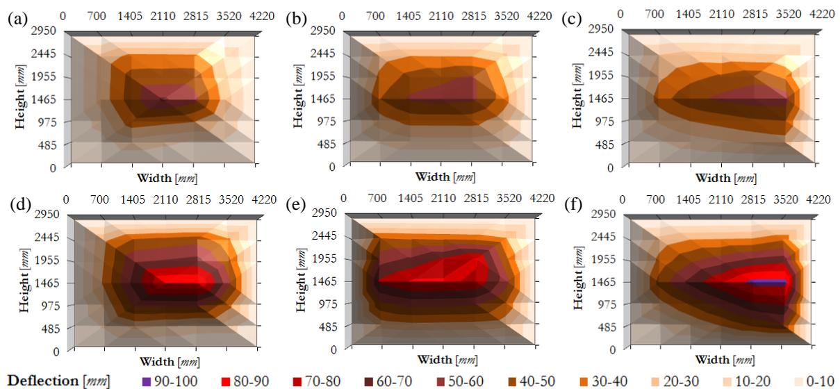
Figure 10. Deflection of fully infilled specimens at 50 mm target displacement: (a) TA2, (b) TA1, (c) TA3 and at 75 mm target displacement: (d) TA2, (e) TA1, (f) TA3
