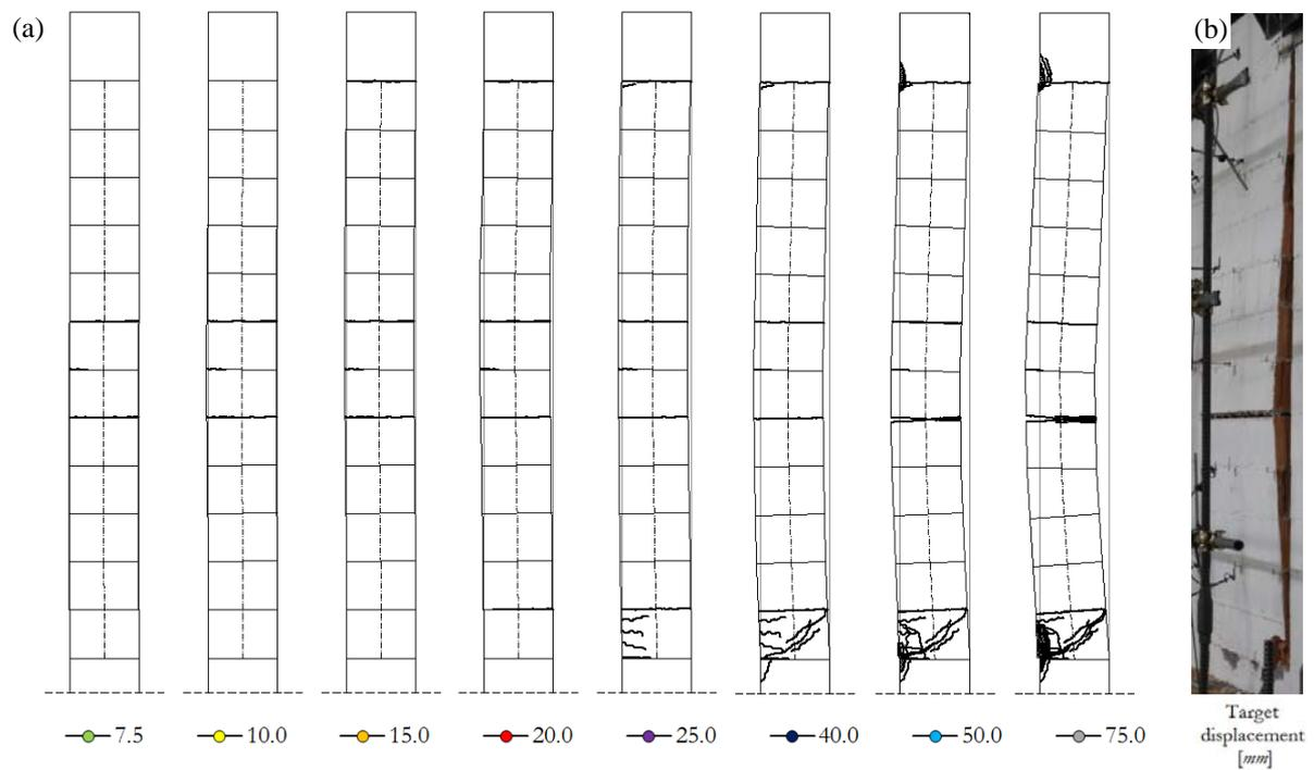
Figure 12. Specimen TA5: (a) Progression of damage; (b) Damage at 75 mm target displacement
