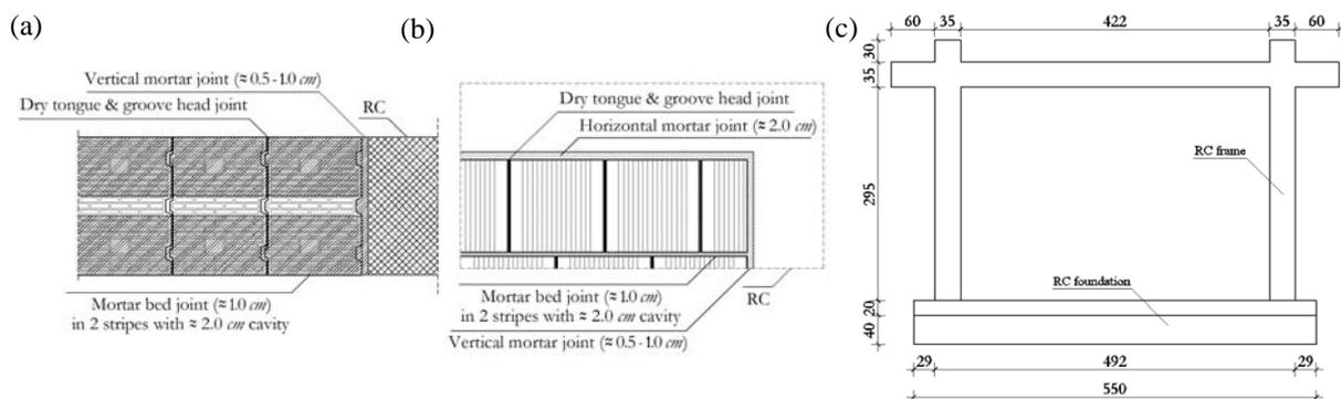
Figure 3. (a) Mortar bed joints; (b) Mortar joints adjacent to RC members; (c) Bare frame
