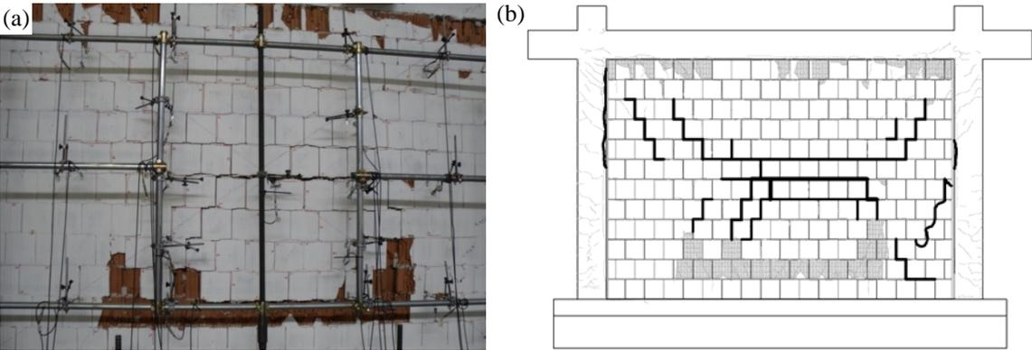
Figure 7. Specimen TA2 (previous in-plane drift: 2.5 %): (a) Damage at  $75\text{ mm}$  target displacement; (b) Crack pattern (in black – out-of-plane damage; in grey – previous in-plane damage)
