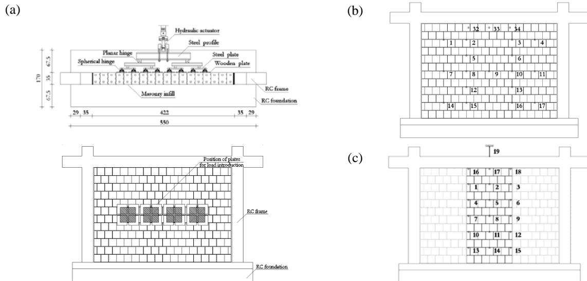
Figure 5. (a) Out-of-plane load transfer system; (b) TA1, TA2, TA3, and (c) TA5 instrumentation layout
