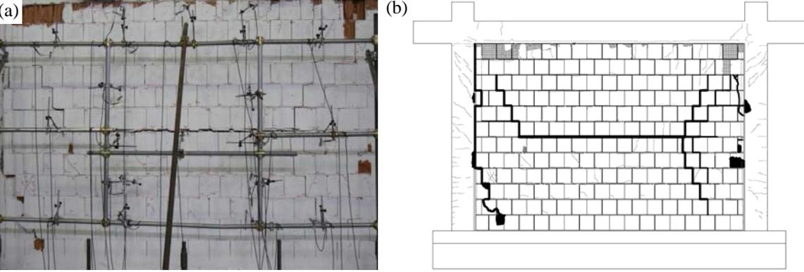
Figure 8. Specimen TA1 (previous in-plane drift: 1.5 %): (a) Damage at  $75\text{ mm}$  target displacement; (b) Crack pattern (in black – out-of-plane damage; in grey – previous in-plane damage)
