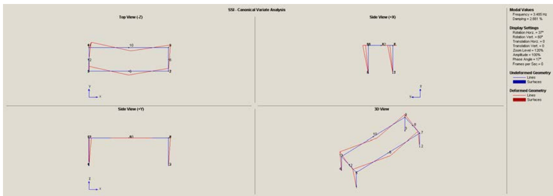
Figure 8. CVA technique – eigenvalue at 3.485 Hz
