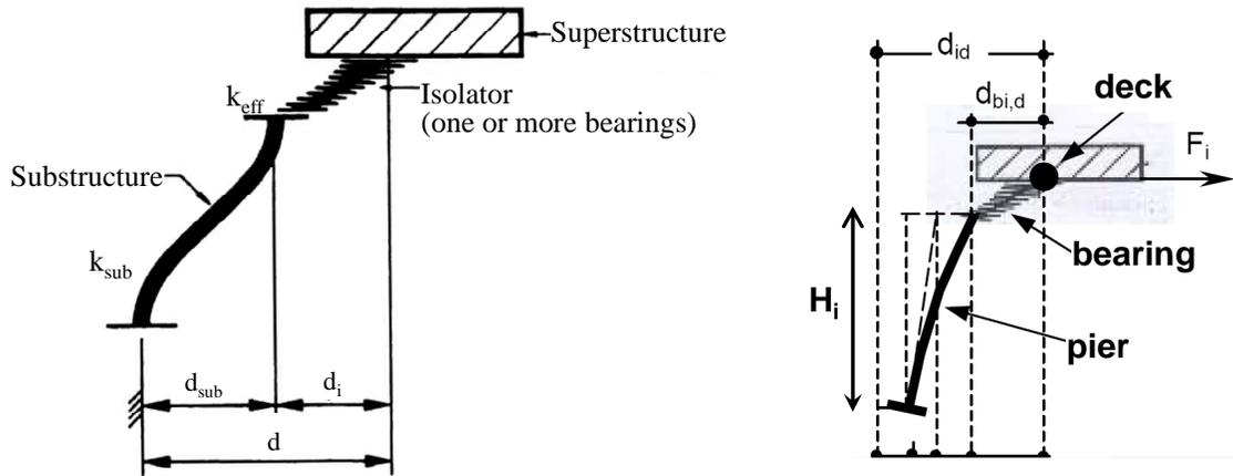
Figure 1. Models of an isolated bridge pier provided in two Standards (a) AASHTO (2010); (b)Eurocode 8 Part 2 (2005).
