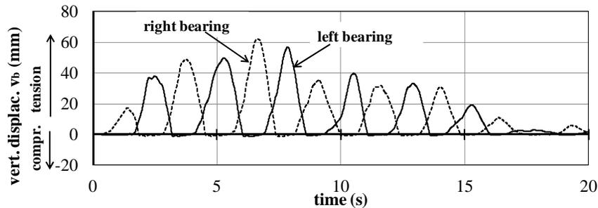
Figure 5. The response of the bearing under axial deflection.
