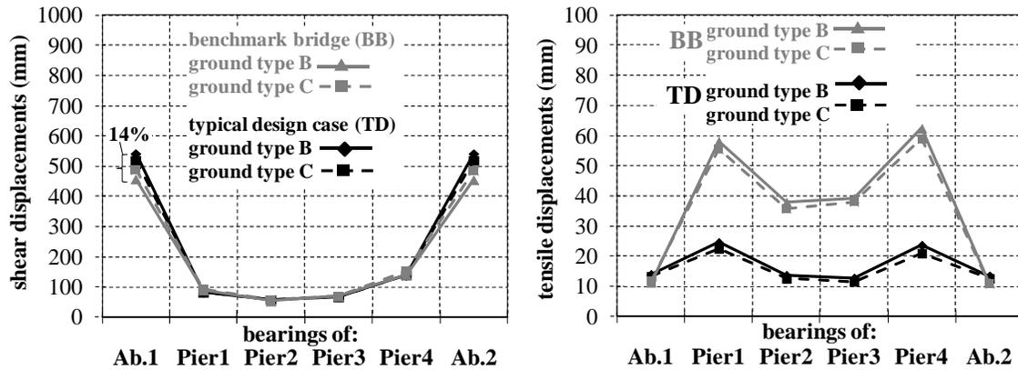
Figure 6. (a) The maximum shear displacements of the BB and the TD bearings at abutment 1, piers 1, 2, 3, 4, abutment 2 and (b) the maximum tensile displacements of the bearings (PGA 0.5g).
