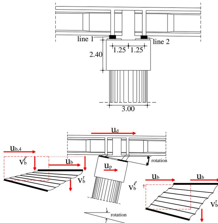
Figure 3. Top figure: the geometry of the pier head and the two lines of support of bearings and bottom figure: the bearings on the left line of support are under compression and the ones on the right are under tension.
