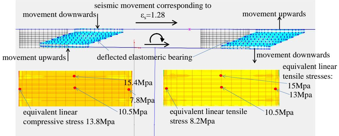
Figure 8. The tensile stress developed at the bearing due to  $\epsilon_s = 128\%$ .
