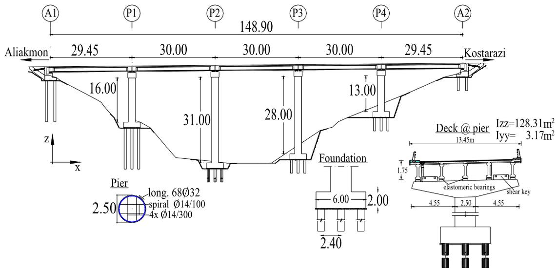
Figure 2. The geometry of the benchmark bridge and cross sections of the pier, the foundation and the deck.
