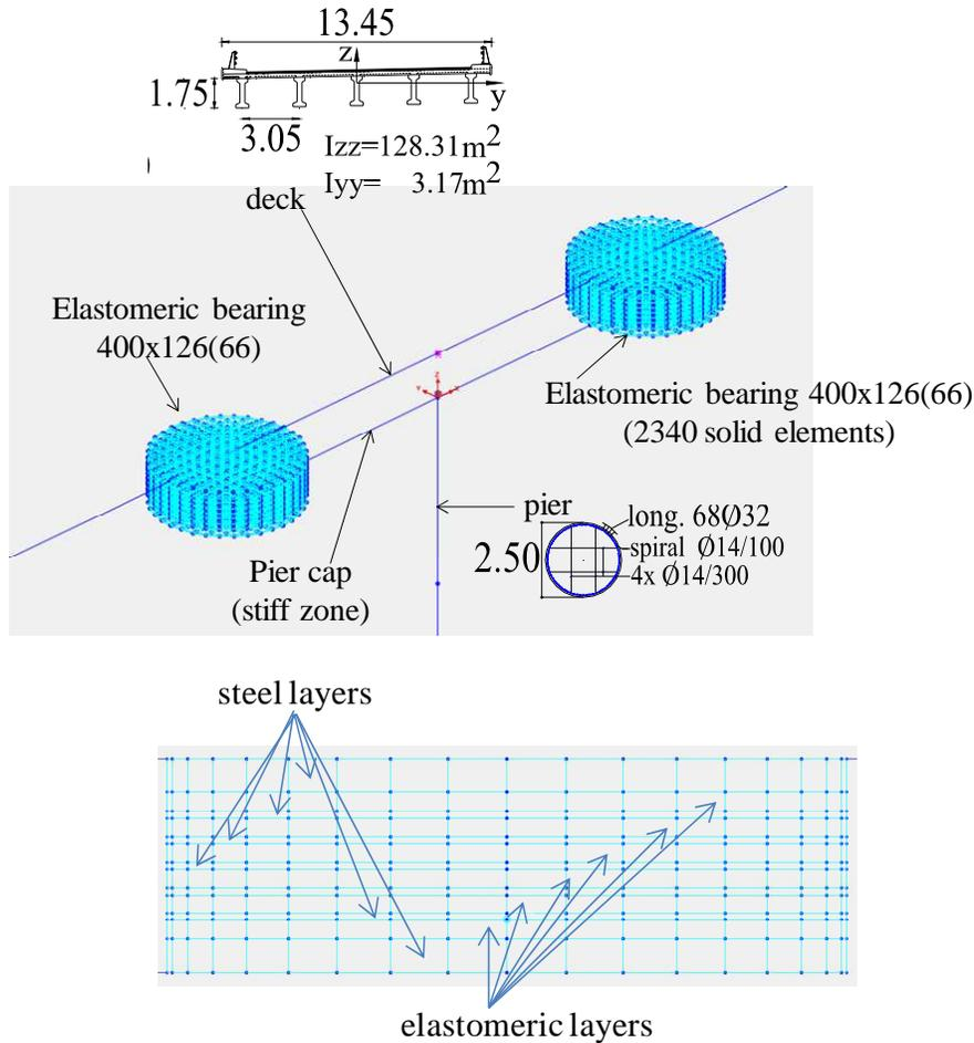
Figure 7. Top figure: A three dimensional representation of the pier - pier cap – bearings - deck connection and bottom figure a cross section of the 3D bearing model.
