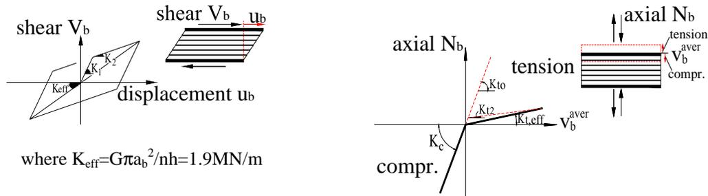
Figure 4. On the left figure: the response of the bearing under shear deflections; on the right: the response of the bearing under axial deflection.
